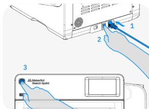
8. Enable power to the machine by using the switch next to the power inlet, then press the power button on the front left of the machine to turn it on.
