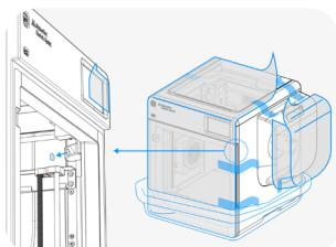
3. Take the printer out of the bag and remove the protective films on the outer panels and on the camera lens inside the build chamber.
