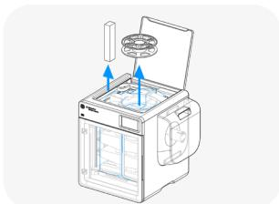
4. Open the top lid and remove the second filament spool and power cords.
