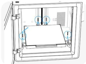
6. Use the 2mm hex key provided to remove 4 screws holding down the Z-stage.
