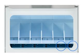
or 2. Push and hold the two right eject buttons This starts the calibration of decoupler 2
