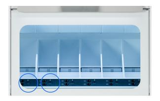
2. Push and hold the two left eject buttons This starts the calibration of decoupler 1
