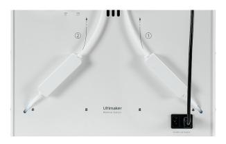
Access the correct decoupler at the back of the Material Station
