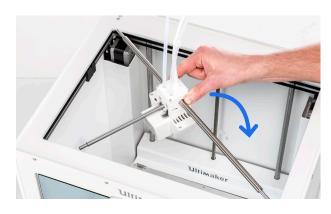
4. Rotate 45° and take the print head out of the printer
