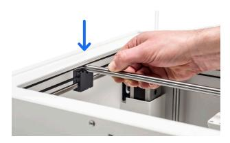
3. Click the ends of the X shaft into the sliding blocks
