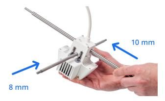
1. Push the print head shafts through the bearings
