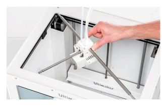
Lower the print head into the printer and align the shafts with the sliding blocks
