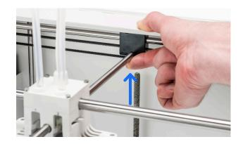
4. Click the ends of the Y shaft into the sliding blocks
