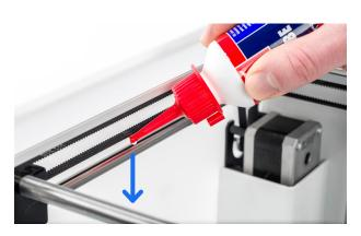
5. Apply a small drop of oil to each shaft and move the print head around to distribute evenly
