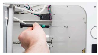
Tip: Place a finger over the locknut while inserting the bolt from the inside of the printer. This ensures that it stays in place.
